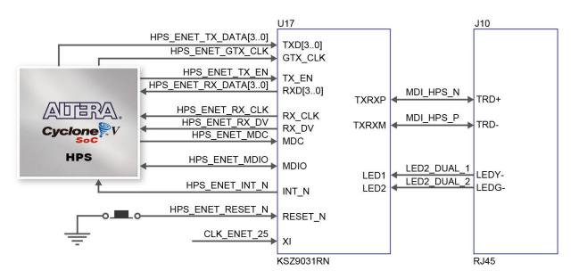
Figure 3-24 Connections between the HPS and Gigabit Ethernet
