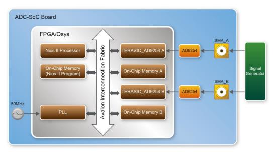
Figure 4-8 Block diagram of Nios II based high-speed ADC demo
