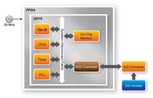
Figure 4-2 Block diagram of ADC reading
