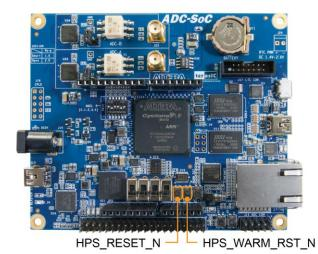
Figure 3-11 HPS cold reset and warm reset buttons on ADC-SoC
