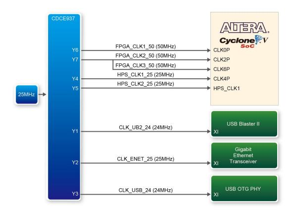
Figure 3-13 Block diagram of the clock distribution on ADC-SoC
