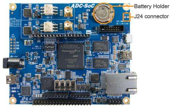
Figure 3-31 battery holder and J24 connector location.
