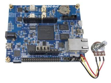
Figure 4-4 Hardware setup for the ADC reading demonstration
