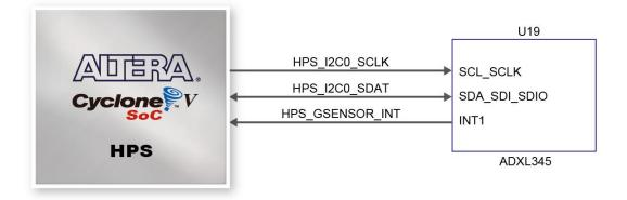
Figure 3-28 Connections between HPS and G-Sensor device.
