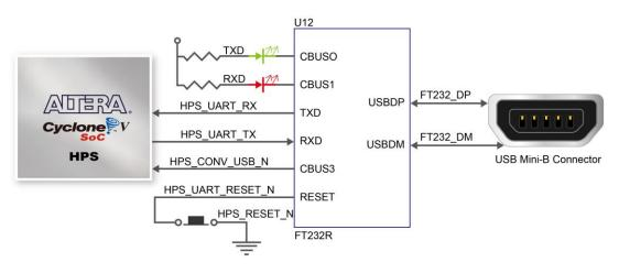
Figure 3-25 Connections between the HPS and FT232R Chip
