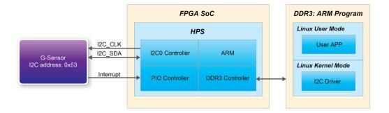
Figure 5-6 Block diagram of the G-sensor demonstration
