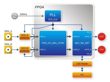
Figure 4-5 Block diagram of HIGH-SPEED-ADC
