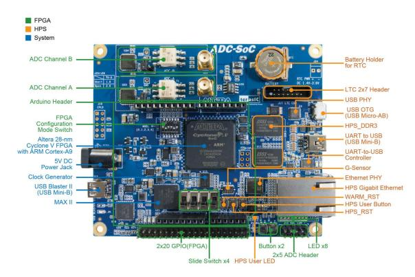
Figure 2-1 ADC-SoC development board (top view)
