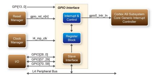
Figure 5-2 Block diagram of GPIO Interface
