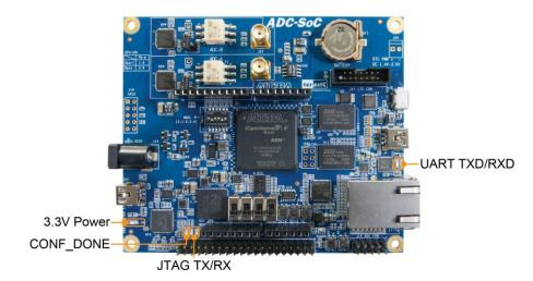
Figure 3-10 LED Indicators on ADC-SoC
