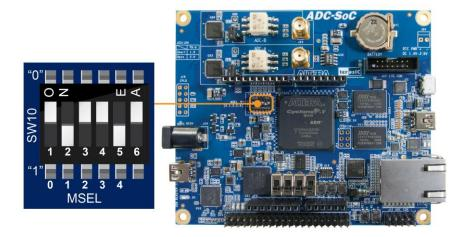
Figure 7-1 DIP switch (SW10) setting of Active Serial (AS) mode
