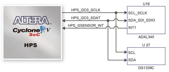
Figure 3-30 Connections between HPS and G-Sensor / RTC device.
