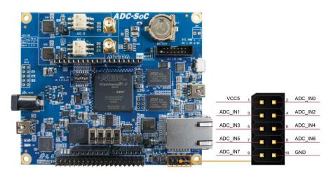
Figure 3-20 Signals of the 2x5 Header
