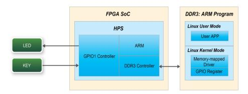
Figure 5-1 Block diagram of GPIO demonstration
