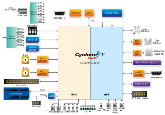
Figure 2-3 Block diagram of ADC-SoC
