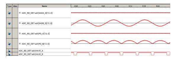
Figure 4-7 SignalTape II viewer for the HIGH-SPEED-ADC
