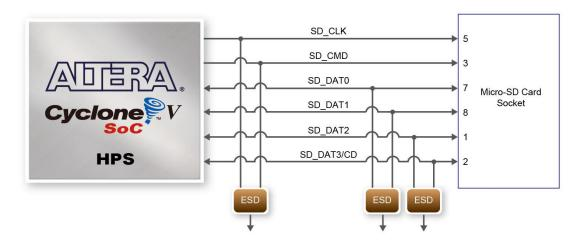
Figure 3-26 Connections between the FPGA and SD card socket
