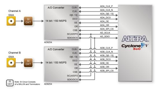
Figure 3-22 Connections between the FPGA and High-Speed ADC.
