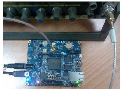
Figure 4-6 Hardware setup for the HIGH-SPEED-ADC
