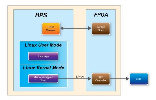
Figure 6-1 FPGA LED are controlled by HPS
