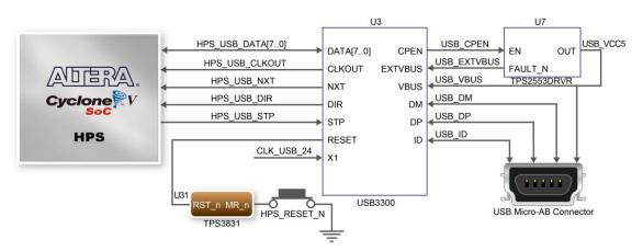
Figure 3-27 Connections between the HPS and USB OTG PHY
