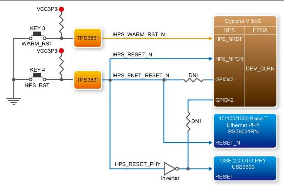
Figure 3-12 HPS reset tree on ADC-SoC board
