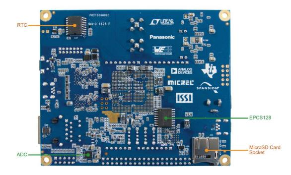
Figure 2-2 ADC-SoC development board (bottom view)
