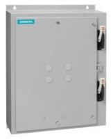
Duplex starter w/ alternator, Size 2, Three phase full voltage, Amb compensate bimetal OLrelay Contactor amp rating 45Amp 110V 50HZ / 120V 60HZ coil, Combination type, Two 60A disconnect switches Enclosure NEMA type 12, Dust/drip proof for indoors
