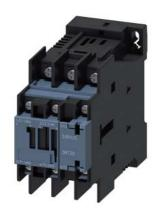
Power contactor, AC-3 38 A, 18.5 kW / 400 V 1 NO + 1 NC, 48 V DC 3-pole, size S0 ring cable lug
