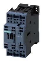
power contactor, AC-3 32 A, 15 kW / 400 V 1 NO + 1 NC, 12 V DC with integrated varistor 3-pole, size S0 spring-type terminal suitable for PLC outputs not expandable with auxiliary switch
