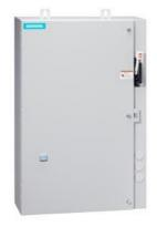
Non-reversing motor starter, Size 2, Three phase full voltage, Solid-state overload relay, OLR amp range 13-52A, Combination type, 60A fusible disconnect, 60A/250V fuse clip, Encl NEMA type 4X 304 S-Steel, Water/dust tight noncorrosive, Extra-wide enclosure
