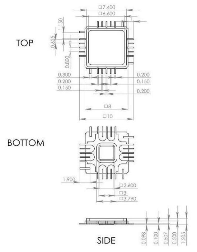
Fig. 4. CQFP 24-Pin Package Drawing (All Dimensions in mm)
