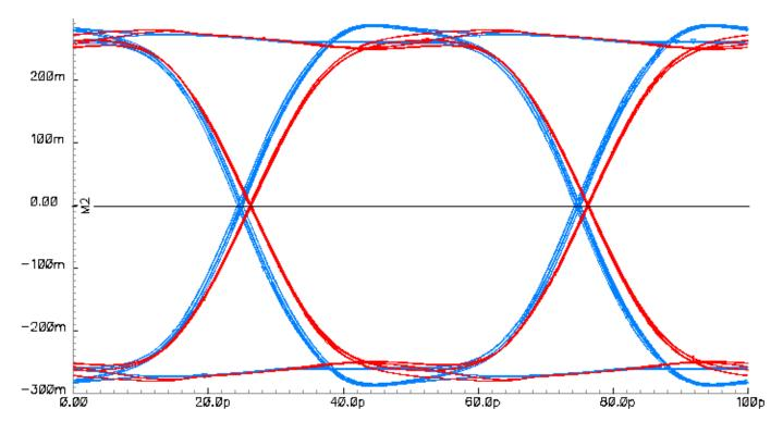
*Fig. 3. 20Gbps PRBS Output Eye Diagram (Simulation, Slow Corner, 125°C)*
