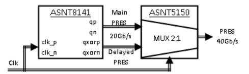
Fig. 2. PRBS Frequency Doubling
