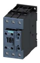
Traction contactor, AC-3 80 A, 37 kW / 400 V 1 NO + 1 NC 110 V DC, 0.7-1.25\* Us with varistor 3-pole, Size S2, screw terminals
