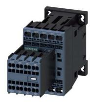
Contactor relay, 6 NO + 2 NC, 24 V DC, Size S00, spring-type terminal, Removable auxiliary switch
