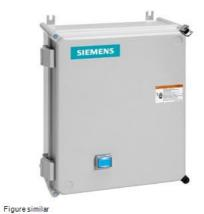
Non-reversing motor starter, Size 1, Single phase full voltage, Solid-state overload relay, OLR amp range 3-12A, 24VAC 50-60Hz coil, Noncombination type, Enclosure type 4X fiberglass, Water/dust tight noncorrosive, Standard width enclosure
