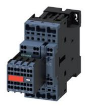
Power contactor, AC-3 25 A, 11 kW / 400 V 2 NO + 2 NC, 24 V DC with plugged-in diode combination, 3-pole, Size S0, Spring type terminal Captive auxiliary switch
