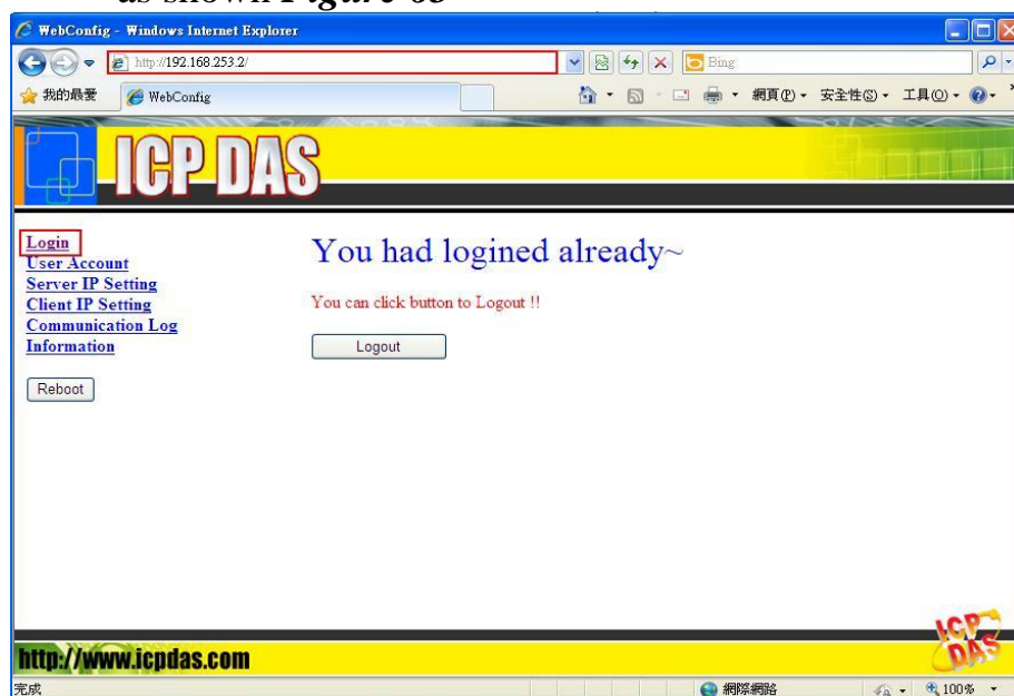
Figure 63 Browse the Web of I-7550E and enter the default password to login.
