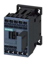
power contactor, AC-3 9 A, 4 kW / 400 V 1 NC, 24 V DC 0.85-1.85\* US, with varistor plugged on, 3-pole, size S00, spring-type terminal not expandable with auxiliary switch
