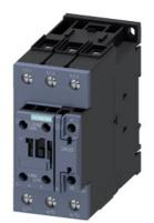
power contactor, AC-3 40 A, 18.5 kW / 400 V 1 NO + 1 NC, 24 V DC with varistor, 3-pole, Size S2, screw terminal Suitable for 2 A PLC outputs
