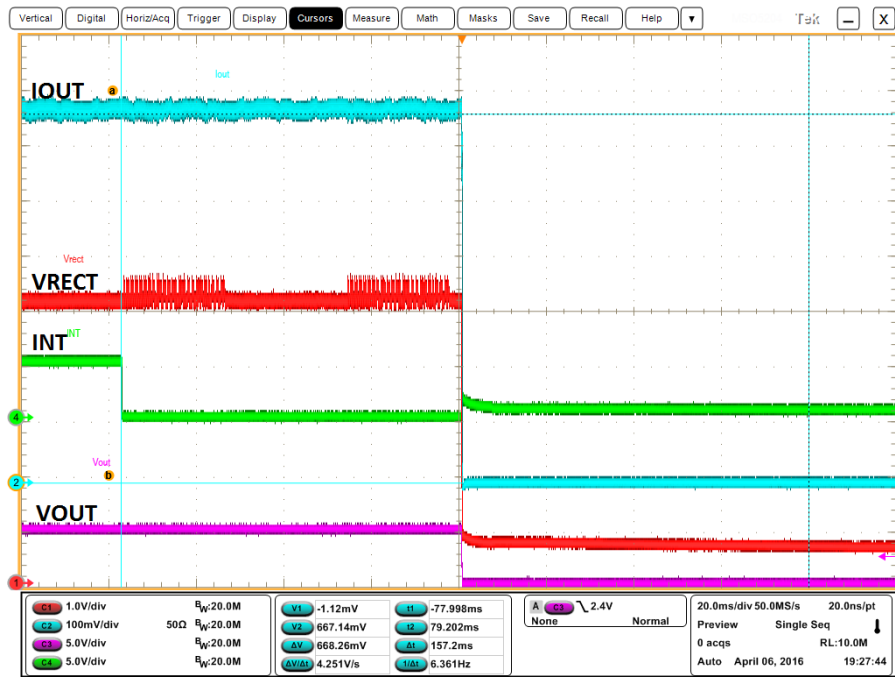
Figure 16. Rx Over Current Protection (Ch1=Vrect, Ch2=Iout, Ch3=Vout, Ch4=INT)
