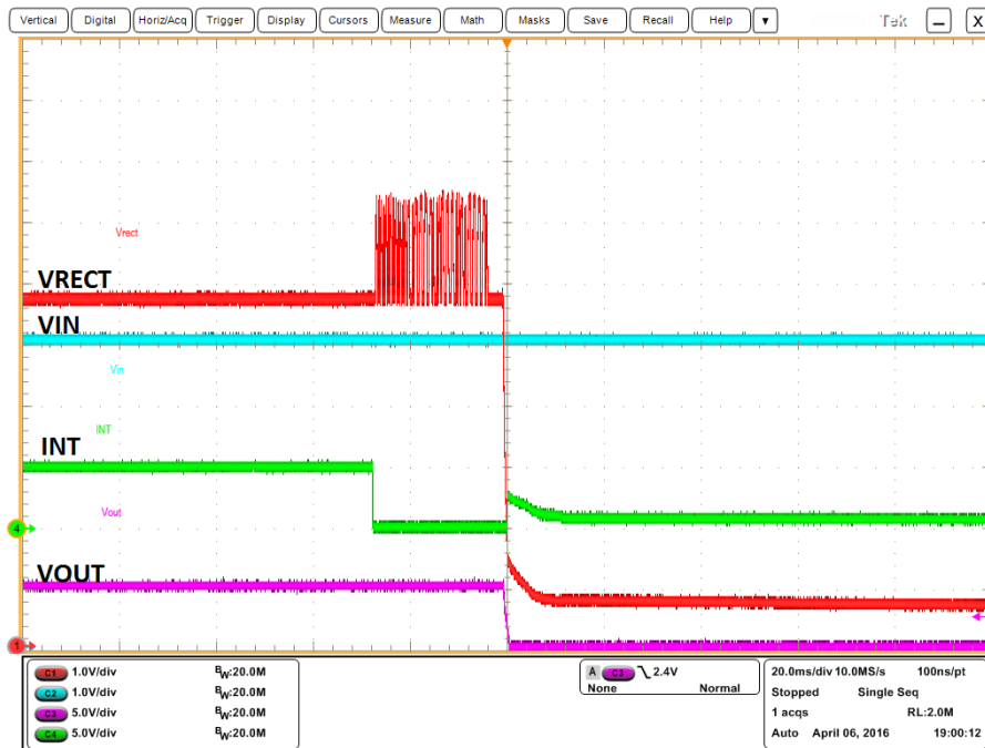
Figure 15. Rx Over Temperature Protection (Ch1=Vrect, Ch2=Vin, Ch3=Vout, Ch4=INT)
