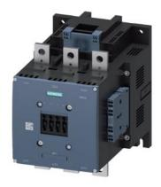
power contactor, AC-3 400 A, 200 kW / 400 V AC (50-60 Hz) / DC operation 220-240 V AC/DC auxiliary contacts 2 NO + 2 NC 3-pole, frame size S12 busbar connections drive: conventional spring-loaded terminal
