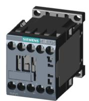
Contactor, 2 NO + 2 NC, AC-3, 5.5 kW, 110 V AC, 50/60 Hz, 4-pole, 2 NO + 2 NC, Size S00, Screw terminal
