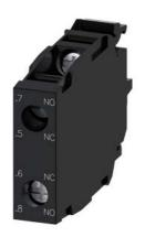
Contact module with 2 contact elements, 1 NO leading + 1 NC lagging, gold-plated contacts, screw terminal, for front plate mounting, Z=150-unit packaging
