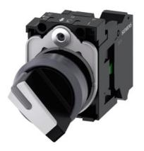
Selector switch, illuminable, 22 mm, round, plastic with metal front ring, white, selector switch, short, 2 switch positions O-I, latching, actuating angle 90°, 10:30h/13:30h, with holder, 1 NO, spring-type terminal, with laser labeling, upper case
