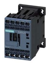
Power contactor, AC-3 16 A, 7.5 kW / 400 V 1 NC, 230 V AC, 50/60 Hz 3-pole, Size S00 Spring-type terminals
