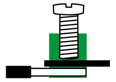
Feed-through terminal, Screw connection, Mounting type: Mounting rail TS 35/7.5, Rated cross-section: 4 mm<sup>2</sup>, Width: 6 mm, Colour: Green
