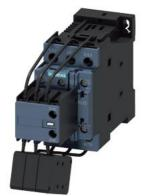
Capacitor contactor, AC-6b 20 kVAr, / 400 V 1 NO + 2 NC, 50-60 Hz AC 21-28 V DC 3-pole, Size S0 screw terminal
