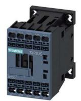
power contactor, AC-3 12 A, 5.5 kW / 400 V 1 NC, 110 V DC, with diode integrated, 3-pole Size S00, Spring-type terminal
