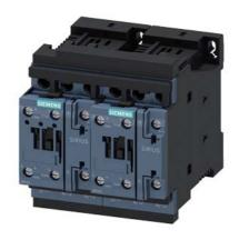
Reversing contactor assembly for 3RA27 AC-3, 5.5~kW/400~V, 24~V~DC~3-pole, Size S0 screw terminal electrical and mechanical interlock 2 NO integrated, with voltage tap
