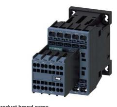
Power contactor, AC-3 7 A, 3 kW / 400 V 2 NO + 2 NC, 110 V AC 50 / 60 Hz, 3-pole, Size S00, Spring-type terminal Removable auxiliary switch
