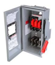
Siemens Low Voltage Circuit Protection Heavy Duty Safety Switch. 3-Pole Non-Fused in a type 3R enclosure (outdoor). Rated 600VAC (60A). Special features: viewing window.
