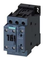
Power contactor, AC-3 38 A, 18.5 kW / 400 V 1 NO + 1 NC AC (50 - 60 Hz) / DC 21-28 V AC / DC, 3-pole Size S0, screw terminals Size S0, screw terminals
