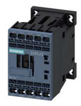
power contactor, AC-3 12 A, 5.5 kW / 400 V 1 NC, 48 V DC 3-pole, Size S00 Spring-type terminal
