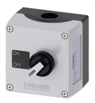
enclosure for command devices 22 mm, round, enclosure material plastic, enclosure top part gray, 1 control point, A= Selector switch, black, plastic, 2 switch positions, latching, label: On Off, 1 NO, 1 NO, screw terminal, floor mounting, 1xM20 each on top and bottom Label glued in
