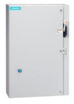
Non-reversing motor starter, Size 2 1/2, Three phase full voltage, Solid-state overload relay, OLR amp range 25-100A, 240V 50Hz / 277V 60Hz coil, Combination type, 60A fusible disconnect, 60A/600V fuse clip, Enclosure NEMA type 1, Indoor general purpose use, Extra-wide enclosure
