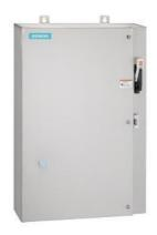
Non-reversing motor starter, Size 3, Three phase full voltage, Solid-state overload relay, OLR amp range 25-100A, 208VAC 60Hz coil, Combination type, 125A circuit breaker, Encl NEMA type 4X 316 S-Steel, Water/dust tight noncorrosive, Extra-wide enclosure
