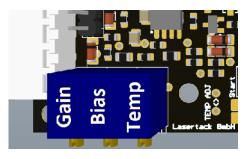
To calculate the needed resistance value for temperature threshold, determine the resistance of the NTC at the threshold temperature in the NTC datasheet. Calculate the required resistance by multiplying the NTC resistance at the threshold temperature by 2,3791.
