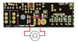
To calculate the hysteresis threshold temperature, divide the previously calculated resistance by 1,7034. This is the Value for the NTC resistance at the hysteresis threshold temperature. The hysteresis temperature is determined with the calculated resistance from the NTC datasheet.
