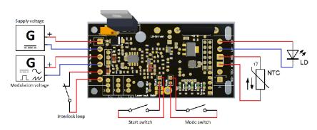
In this mode the driver starts with a power-up delay and will wait for a start signal afterwards, if the remaining start conditions are fulfilled.
