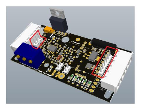
Plug the connectors of the TEC board into the corresponding connectors on the mainboard. Pay attention on not to reverse connection. Plug the short socket onto the short pin strip and the long socket onto the long pin strip.
