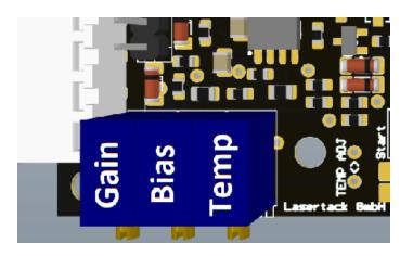
To calculate the needed resistance value for temperature threshold, determine the resistance of the NTC at the threshold temperature in the NTC datasheet. Calculate the needed resistance by multiply the NTC resistance at the threshold temperature by 2,3791.
