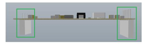
These sockets fit the marked pin strips on the driver board.
