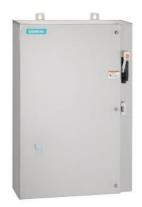
Non-reversing motor starter, Size 4, Three phase full voltage, Solid-state overload relay, OLR amp range 50-200A, Combination type, 150A circuit breaker, Encl NEMA type 4X 316 S-Steel, Water/dust tight noncorrosive, Standard width enclosure
