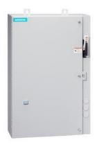
Non-reversing motor starter, Size 1, Three phase full voltage, Solid-state overload relay, OLR amp range 0.75-3.4A, Combination type, 30A fusible disconnect, 30A/600V fuse clip, Enclosure NEMA type 4/12, Water/dust tight for outdoors, Extra-wide enclosure
