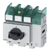
SENTRON, Molded case switch 3LD5 UL, Main switch, 4-pole, certified according to UL489 UL60947-4-1 and IEC60947-3, UL: 60A, SCCR 50kA at 480VAC, Operating power at 480VAC 3-phase: 40hp, IEC: 63A, Operating power at AC-23A at 400V: 30kW, floor mounting with direct handle, black, incl. terminal covers for the infeed side
