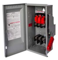
Siemens Low Voltage Circuit Protection Heavy Duty Safety Switch. 3-Pole Non-Fused in a type 3R enclosure (outdoor). Rated 600VAC (30A). Special features: viewing window.
