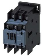
power contactor, AC-3 25 A, 11 kW / 400 V 1 NO + 1 NC, 400 V AC, 50 Hz, 400-440 V, 60 Hz, 3-pole, Size S0, ring cable lug connection
