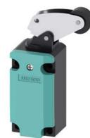
Position switch Plastic enclosure 40 mm according to EN 50041 Device connection  $1x (M20 \times 1.5) 1 \text{ NO}/1 \text{ NC}$  slow-action contacts Angular roller lever made of metal and plastic roller 22 mm
