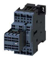
Power contactor, AC-3 32 A, 15 kW / 400 V 2 NO + 2 NC, 110 V DC 3-pole, size S0 Spring-type terminals Removable auxiliary switch
