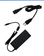
Use only the power cord provided with the unit (4 ft - 1.2m) or equivalent UL approved type SPT-2, SVT, or SJT 18/3 AWG 100-240 VAC, 1 Amp 60°C:
