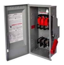
Siemens Low Voltage Circuit Protection Heavy Duty Safety Switches. Type: ENCLOSED, SAFETY SWITCH Std: UL V. Rating: 600V A. Rating: 100A Wattage: 3W No. Of Poles: 3P F. Rating: 60Hz Action: SINGLE THROW Material: STEEL Enclosure: TYPE 1. 2-3 point mounting holes. O. Cycles: 10000 O. Temperature: (-20F-120F) AMBIENT TEMPERATURE Environmental Conditions: INDOOR
