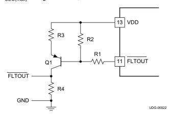
Figure 9. Interfacing to FLTOUT
