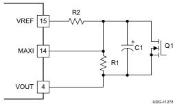
Figure 4. Soft-Start Circuit Using A Higher-Cost Bi-**Polar Transistor**
