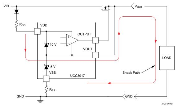
Figure 10. Simplified Schematic Illustrating IDD Sneak Path
