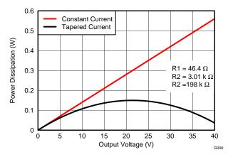
Figure 12. Output Voltage vs. Power Dissipation
