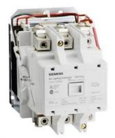
Mechanically held lighting contactor, Contactor amp rating 100A, 0 N.C. / 5 N.O. poles, 220VAC 50HZ/240VAC 60HZ coil, Non-combination type, Enclosure NEMA type (open), No enclosure
