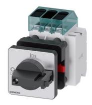
Load disconnector 3LD3, lu 40 A Main switch 3-pole Rated operating capacity at AC-23 A at 400 V 18.5 kW Front plate mounting Basic switch with Central hole mounting 22.5mm Toggle drive black 48x48 mm with auxiliary switch 1OE + 1S
