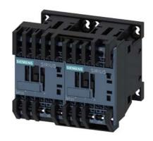
Reversing contactor assembly AC-3,4 kW/400 V,AC230V,50/60 Hz 3-pole, Size S00 Spring-type terminal electrical and mechanical interlock
