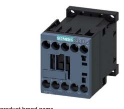
Power contactor, AC-3 12 A, 5.5 kW / 400 V 1 NO, 220 V AC, 50 / 60 Hz 3-pole, Size S00 screw terminal
