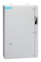
Non-reversing motor starter, Size 0, Three phase full voltage, Solid-state overload relay, OLR amp range 0.75-3.4A, 24VDC coil, Combination type, 30A non-fusible disconnect, Encl NEMA type 4X 304 S-Steel, Water/dust tight noncorrosive, Extra-wide enclosure
