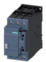
Capacitor contactor, AC-6b 50 kVAr, / 400 V 1 NO + 1 NC, 230 V AC, 50 Hz 3-pole, Size S2 screw terminal
