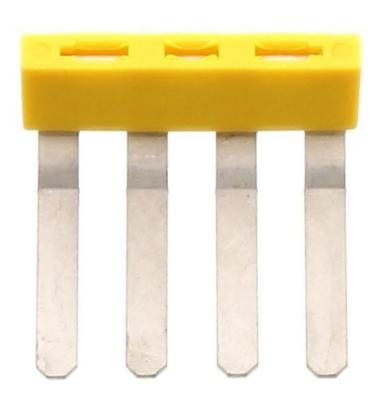
External insulated cross-connector, No. of poles: 4, Mounting type: Plug in, Width: 23 mm, Rated current: 27 A; Colour: Yellow
