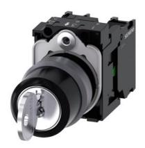
RONIS key-operated switch, 22 mm, round, plastic with metal front ring, lock number SB30, with 2 keys, 3 switch positions I-O-II, latching, actuating angle 2x45°, 10:30h/12h/13:30h, Key removal I+O+II, with holder, 1 NO, 1 NO, screw terminal, possible special locks: SB31, 421, 455, with laser labeling, lower case
