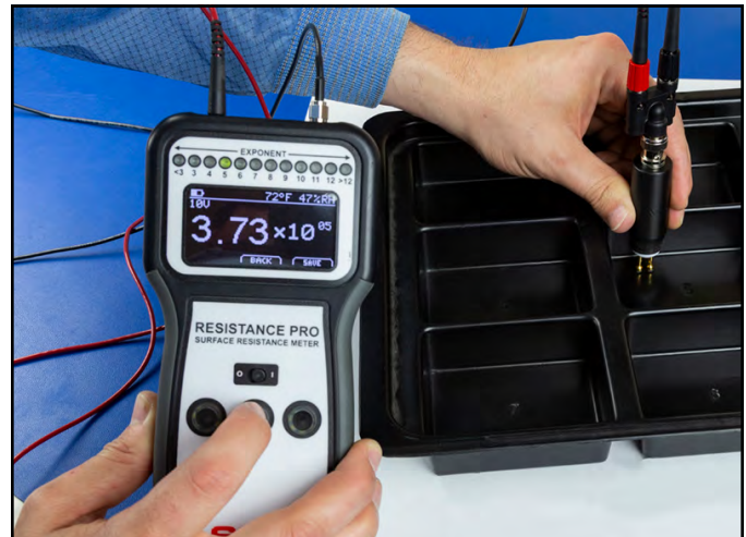
Figure 2. Using the Two-Point Resistance Probe with the SCS 770760 Resistance Pro Meter Kit
